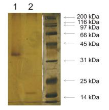
Figure 1. SDS polyacrylamide electrophoresis (12 %, Tris-glycine, pH 8,8 electrode buffer) of nuclease from black pine pollen (PN). Purified sample under non-reducing (without dithiotreitol), (Line1) and reducing (with dithiotreitol) condition (Line2).
