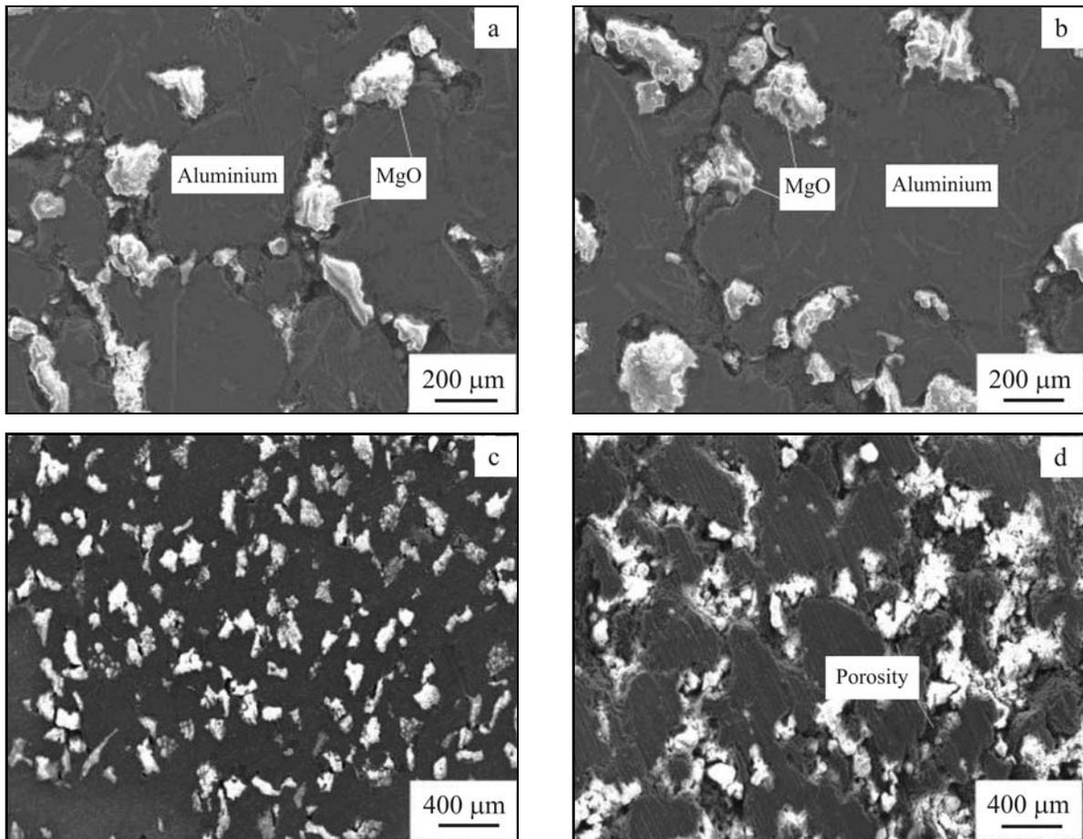
Fig. 3. Microstructure of the produced composites for different amounts of reinforcement phase: (a) Al-10vol.%MgO, (b) Al-20vol.%MgO, (c) Al-30vol.%MgO and (d) Al-40vol.%MgO.
