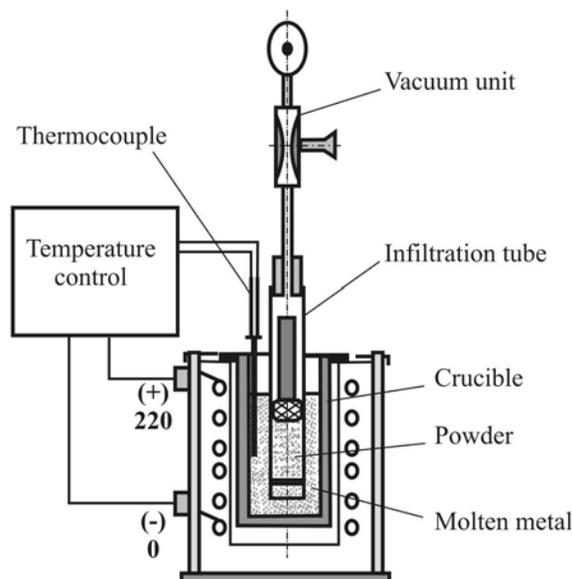
Fig. 1. Vacuum infiltration apparatus.
