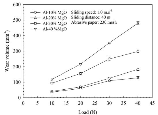
Fig. 8. Wear volume of the produced composites as a function of applied load.
