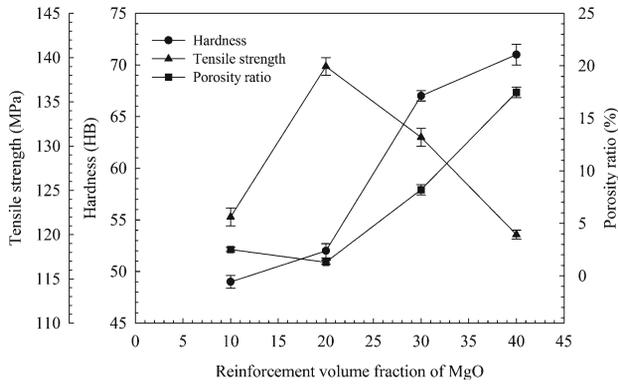
Fig. 4. Variation of hardness, tensile strength and porosity of the produced composites as a function of MgO contents.
