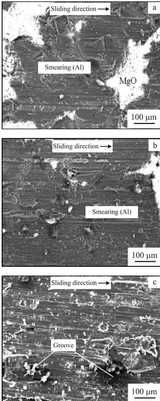
Fig. 11. SEM images of the worn surfaces of the Al-20%MgO composite tested at different loads: (a) 10 N, (b) 20 N and (c) 30 N at a sliding speed of  $1 \text{ m s}^{-1}$  for a sliding distance of 40 m.
