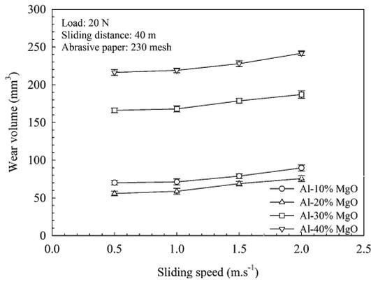
Fig. 9. Wear volume of the produced composites as a function of sliding speed.
