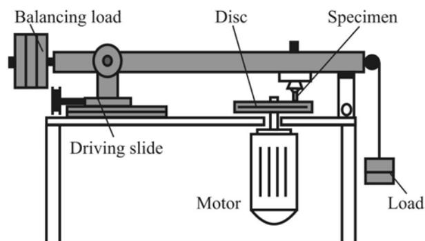
Fig. 2. Schematic diagram of the used wear test machine.
