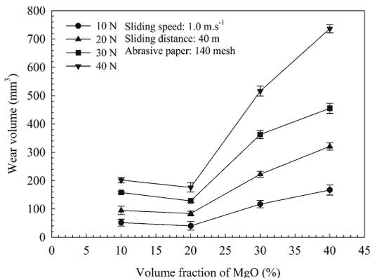
Fig. 5. Wear volume as a function of MgO volume fraction using 140 mesh abrasive paper.
