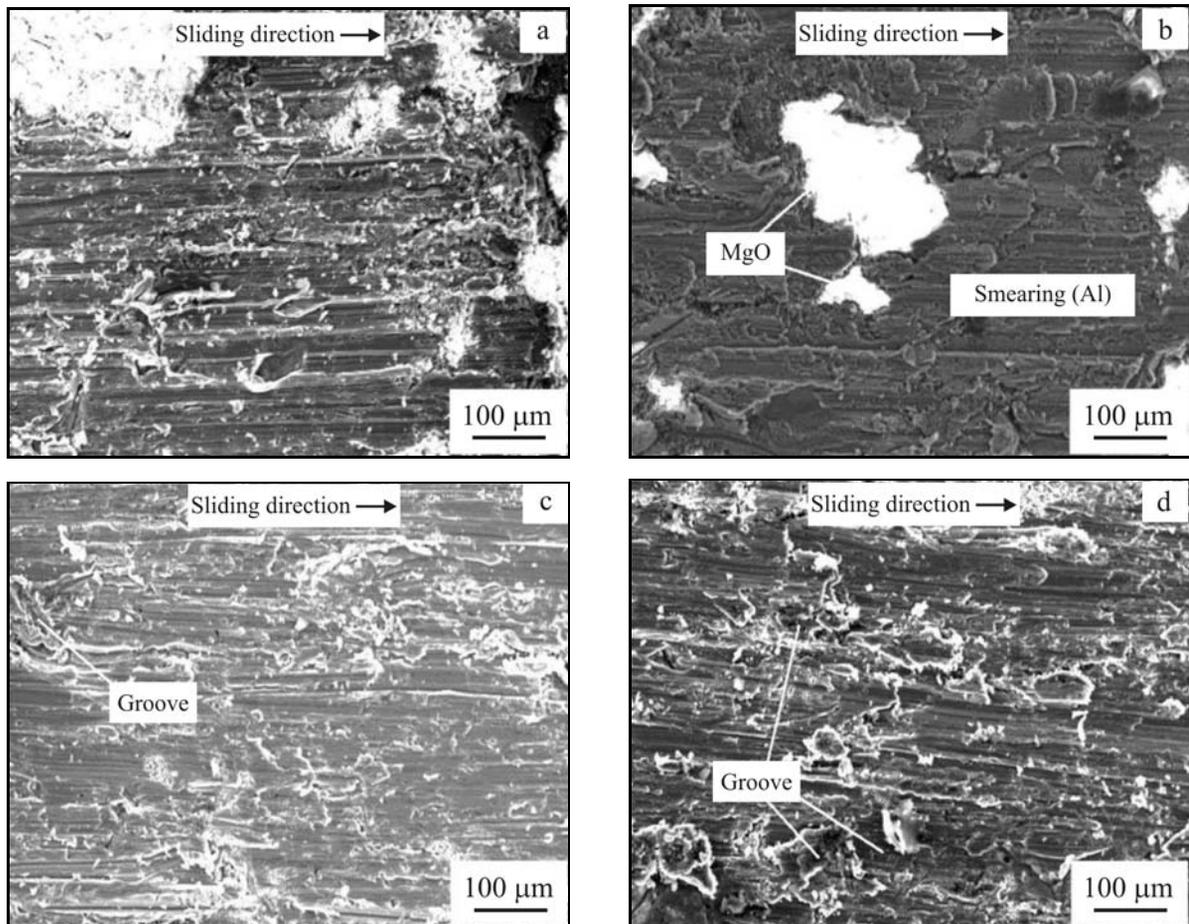
Fig. 10. Wear surfaces of (a) Al-10%MgO, (b) Al-20%MgO, (c) Al-30%MgO and (d) Al-40%MgO composites tested at a load of 20 N and a speed of 1.0 m s<sup>-1</sup> for a sliding distance of 40 m.
