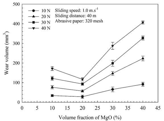
Fig. 7. Wear volume as a function of MgO volume fraction using 320 mesh abrasive paper.
