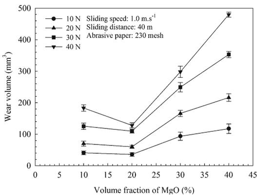
Fig. 6. Wear volume as a function of MgO volume fraction using 230 mesh abrasive paper.
