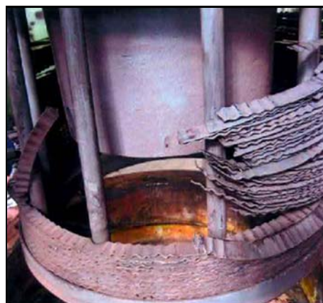
Fig. 1. An image of the damaged separator.
