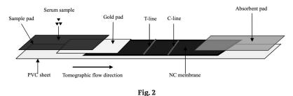
Schematic representation of the structure of CGIA strip for the detection of anti-ASFV antibody
