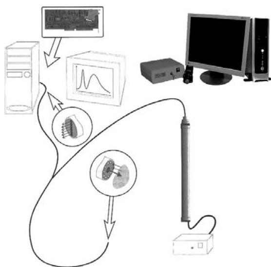
Figure 1. Scheme and photography of LESA-01-BIOSPEC.
