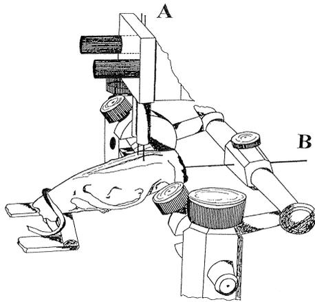
**Fig. 1.** Position of a rat skull in a stereotaxic instrument adapted for perfusion of cerebral ventricles. A- inflow cannulae for lateral ventricles, B – outflow cannula for cerebellomedullary cistern.
